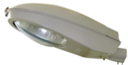
1. Street Lighting STA-100/150/250/315W Casing Dimension 910 x 360 x 210 ø64 (mm) Weight : 8 / 8.7 kg IP65
