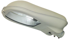
3.Ndricim Rrugor STK-70/100/150/250W Dimensioni I Kutise 650x 350x 210 ø60 (mm) Pesha : 7.5 Kg IP65
